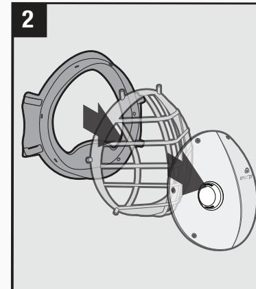
Pull filter from the respirator body. Remove filter from filter cage and dispose of the filter. Follow **Respirator Assembly** instructions to reassemble.
