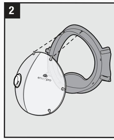
Take the assembled filter cage and insert the posts into the respirator body. Make sure to start with the top two posts.
