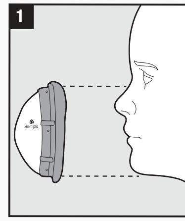
Make sure the top of the respirator rests on the bridge of the nose and the bottom flap rests on the chin.
