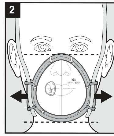
Pull the straps on both sides of the respirator body to adjust and balance.
