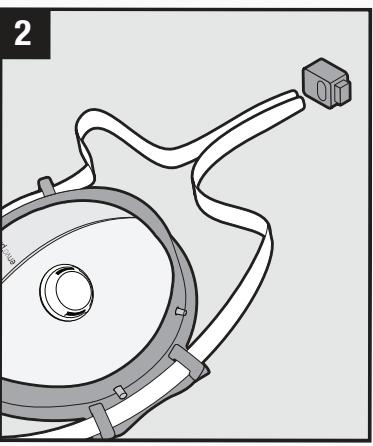
Once the threads have passed through, align the straps and reassemble the cordlock.
