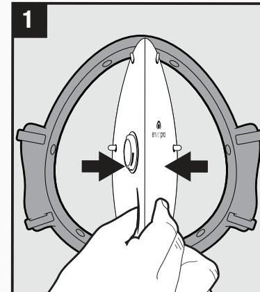
Squeeze the filter to remove it from the respirator body.
