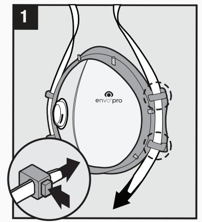
Remove cord lock from the strap. Thread both tapered ends through the headgear slots from the top of the envo® pro.
