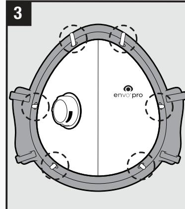
Place the rest of the posts in the respirator body holes. Check to make sure that all of the posts are sticking out.
